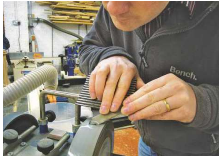
▲ Pic 9 He ground an edge into the blade with a general mounting jig set at 25°...
